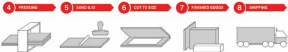
The fabrication process involves pressing, sanding, cutting, finishing, and shipping to final users.
