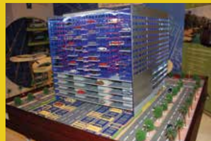
APSs do not need to accommodate people driving cars with ramps and elevators and lighting. The robotic machinery and sophisticated software do the job. This model shows a conventional garage on the bottom with automatic parking above.
