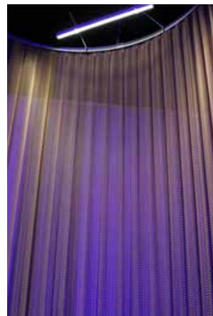
Attachment systems for coiled wire fabric are typically based on frames or tracks that can be designed to suit different shapes, sizes, and installations.
