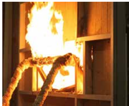
Shown here is mullion exposure to fire during testing. Note that the exposed side of the vertical mullion is almost completely melted out.
