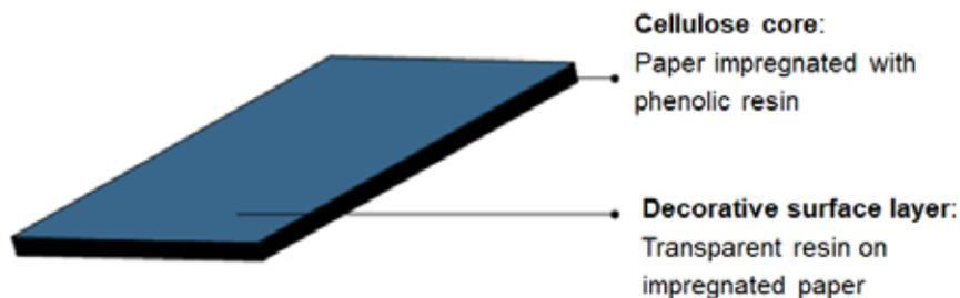
**HPL is made up of a core of multiple layers of resin-impregnated kraft paper, plus outer surface layers that are decorative or colored.**
