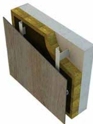
**A ventilated rainscreen facade incorporates an outer cladding material held out from the wall assembly with an aluminum support system. It also allows for continuous insulation and a water-resistant barrier (WRB) to be properly installed.**
