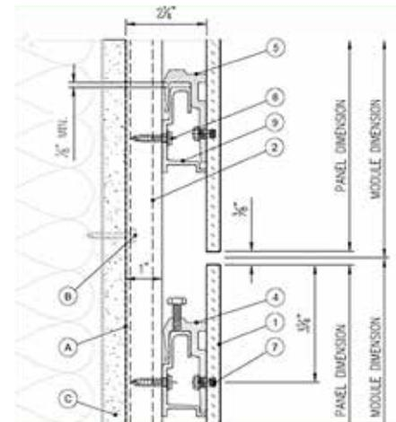
HPL panels can be installed on aluminum support systems using either an exposed fastener method or concealed fastener system.
