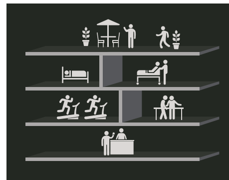
Noise generated within a building includes walking, exercise, rolling carts, etc.
